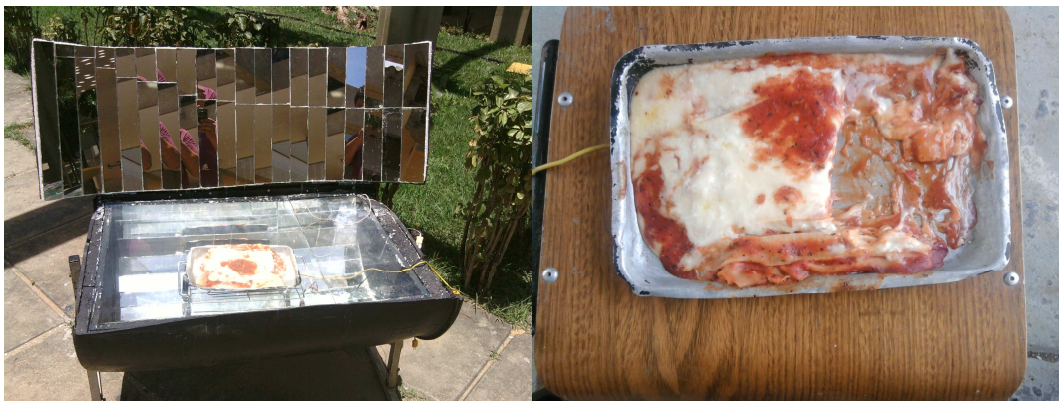
Figure 8. Solar oven/cooker modified test for baking a lasagna and baked lasagna after.
