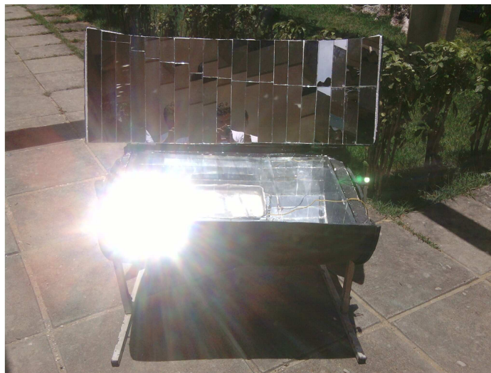
Figure 3. Solar oven/cooker in its design modified.
