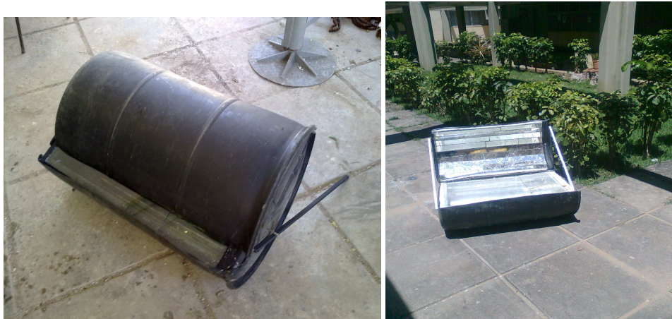
Figure 2. Solar oven / cooker in his first design.
