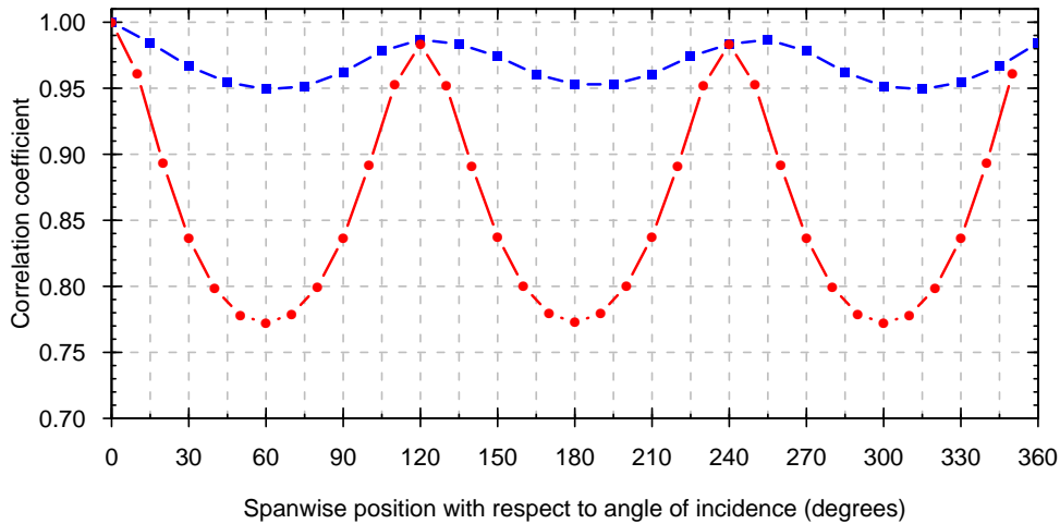
Figure 5. Correlation coefficient C from Eq. 9. Red circles line: current computational simulation; Blue squares line: experimental from PIV in Korkischko and Meneghini (2011).
