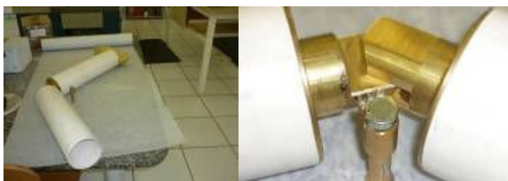
Figure 16. Additional angular position sensor to be installed on the prosthesis.
