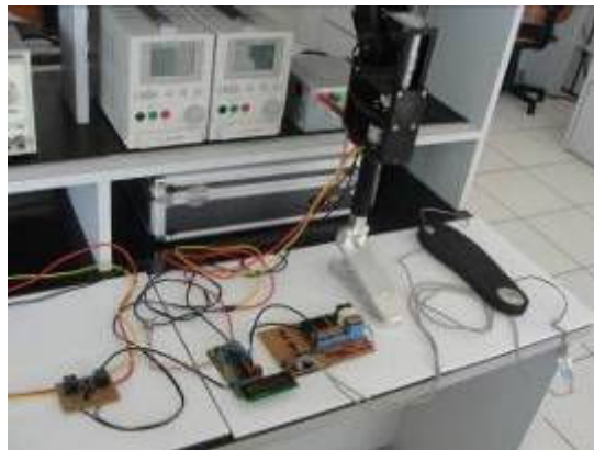
Figure 15. Apparatus to test the prosthesis components.
