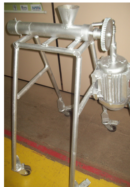
Figure 12 and 13. Photo of the prototype of the screw press.
