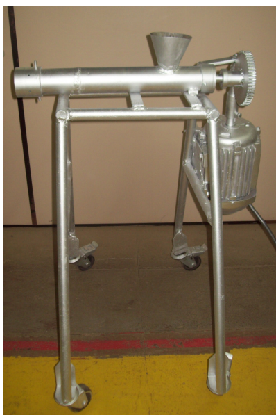
Figure 12 and 13. Photo of the prototype of the screw press.
