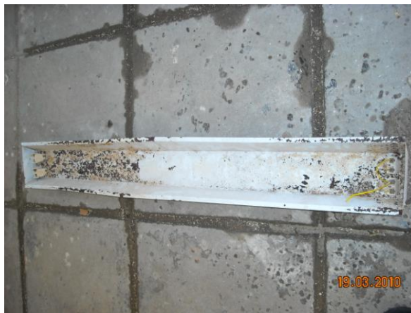
Figure 2. Scrap lamp used as a template to construct the proposed solar dryer.
