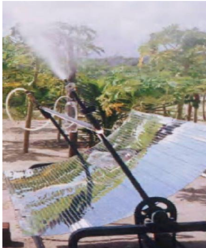
Figure 5. Cylinder-parabolic solar concentrator to be used on the refrigeration cycle for the studied refrigerator.
