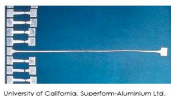
Fig. 3 - Aluminum alloy EN AW 7475 superplastic forming (Robert, 2009)
