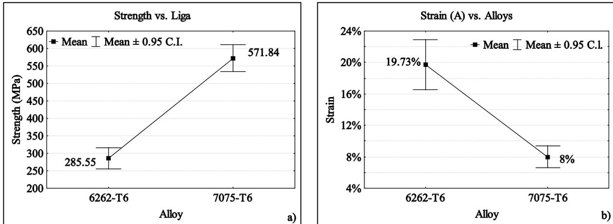
Figure 2. a) Ultimate tensile strength and b) Elongation of the 6262-T6 and 7075-T6 aluminum alloys
