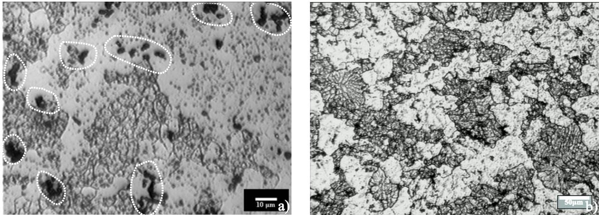
Figure 3. a) Microstructure of the 6262-T6 aluminum alloy: b) Microstructure of the alloy 7075-T6 aluminum
