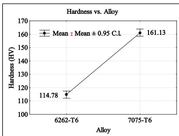
Figure 1. Mean hardness of aluminum alloys
