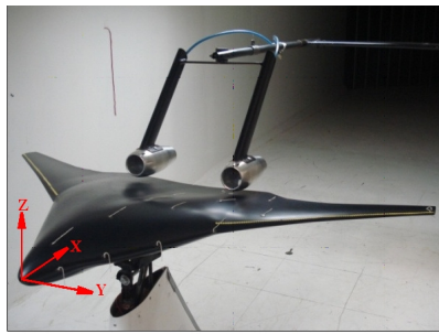
Figure 6. BWB model inside the working section
