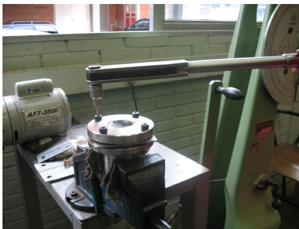
Figure 3. Torque meter used to normalize the pressure applied on the welding sample before the formability test
