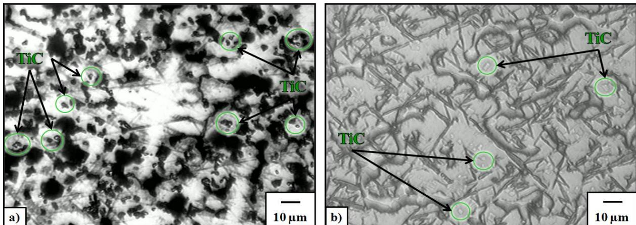
Figure 7. Microstructure of FeCr+ Ti alloy : a) etched with kalling for 10 seconds and b) etched with Murakami at 60°C for 10 seconds.
