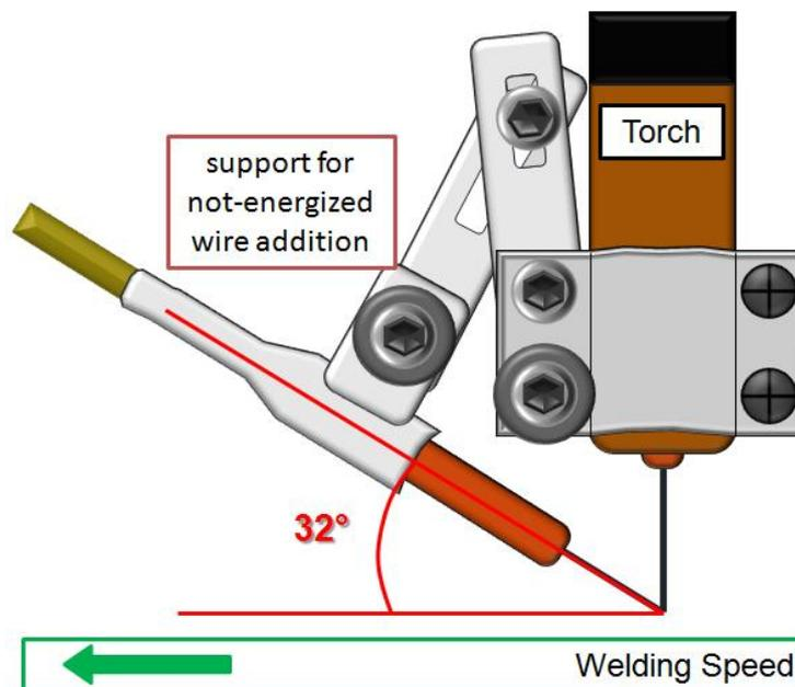
Figure 1. Support for addition of the wire not energized.
