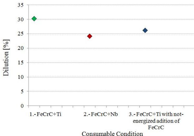
Figure 3. Mean values of dilution of the hardfacing condition.
