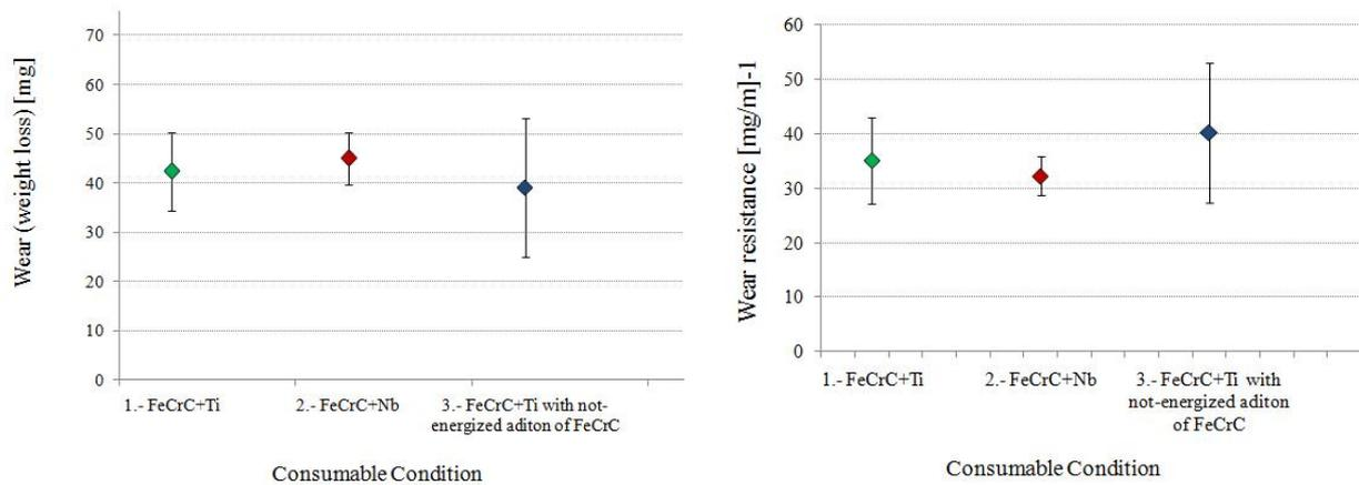
Figure 4. Analysis comparative of wear resistance.
