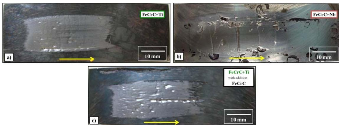
Figure 5. Test piece wear strips for each consumable: a) FeCrC+Nb, b) FeCrC+Ti and c) FeCrC+Ti with addition wire not energized of FeCrC.
