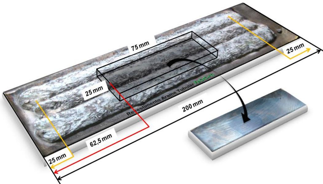
Figure 2. Test plate and region of the test specimen for wear and microstructure evaluation.
