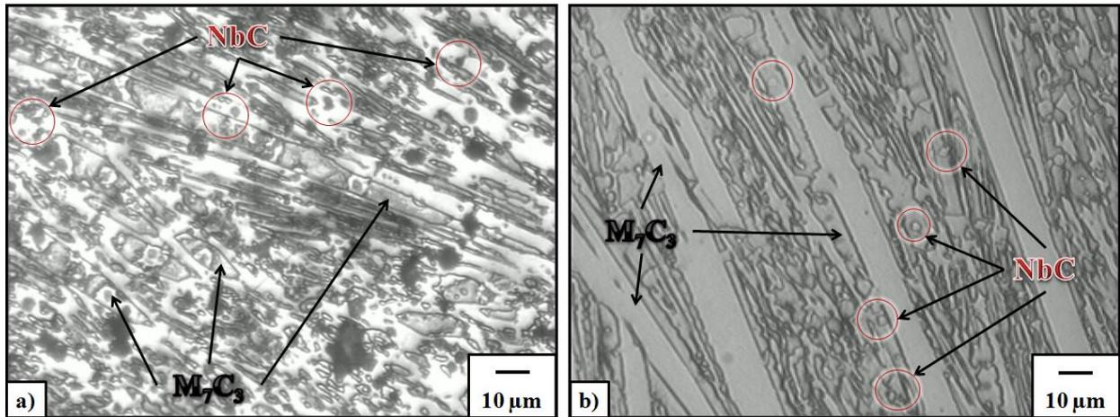
Figure 6. Microstructure of FeCr+ Nb alloy: a) etched with kalling for 10 seconds and b) etched with Murakami at 60°C for 10 seconds.
