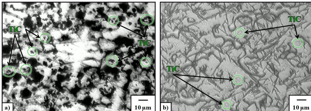
Figure 8. Microstructure of FeCrC+Ti alloy with wire not energized FeCrC. : a) etched with kalling for 10 seconds and b) etched with Murakami at 60°C for 10 seconds.
