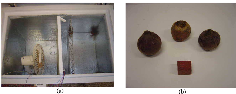
Figure 5. (a) Internal arrangement of the freezer with a three-dimensional sample of beets ready for the freezing. (b) Sample parallelepiped-shaped bulbs beets.
