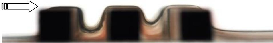
Figure 3. Low velocity test in  $Re \cong 5$  shows a stable flow in very low velocity.
