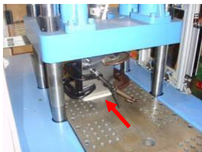
Figure 13. Tape being used to place the insert on the injection table
