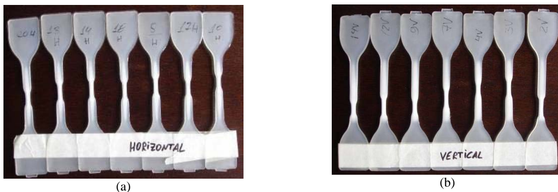
Figure 20. Horizontal (a) and vertical (b) tensile test specimens after tests
