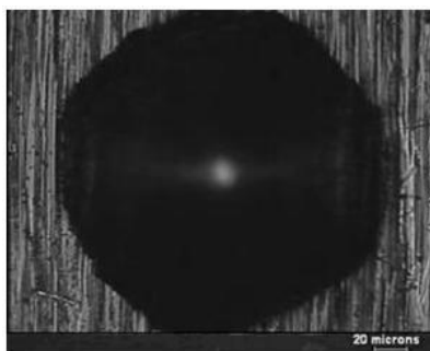
Figure 6. Adherence test by penetration, using the Revetest equipment to a constant load of 50 N.
