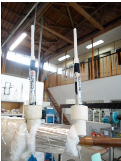
Figure 2. Two SPME devices inserted through septum in the gas sampling piping.
