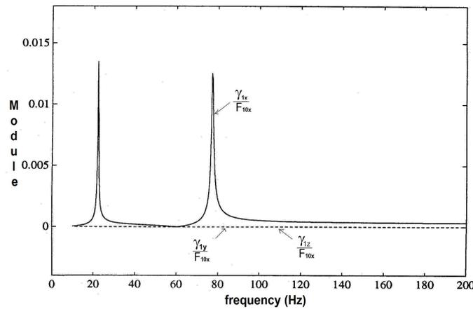
Figure 5. Transfer function at node 1 - Junction (without parasite motion)
