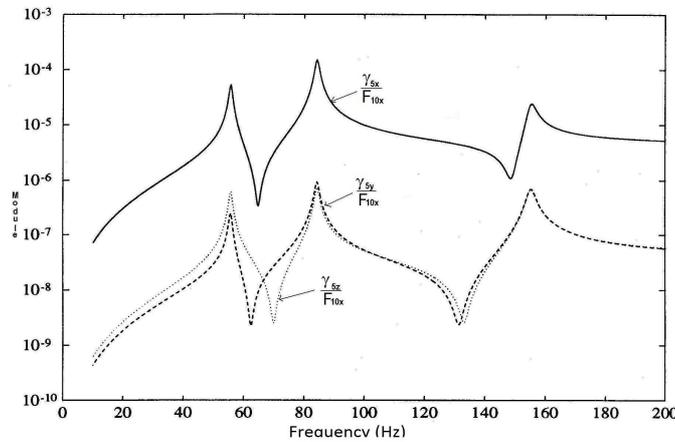
Figure 6. Transfer function at node 5 - Interne (without parasite motion)
