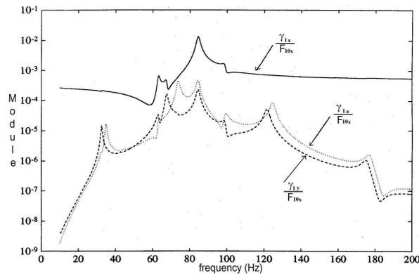
Figure 3. Transfer function at node 1 - Junction (with residual terms)
