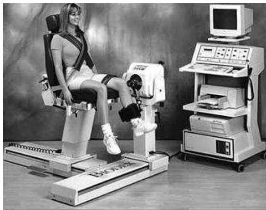
Figure 1. Isokinetic device with torque generator Calota et al. (2008).
