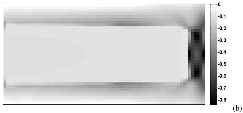
Figure 5. Bending load case. (a) Convergence history of the objective function, (b) \epsilon -relaxed failure function
