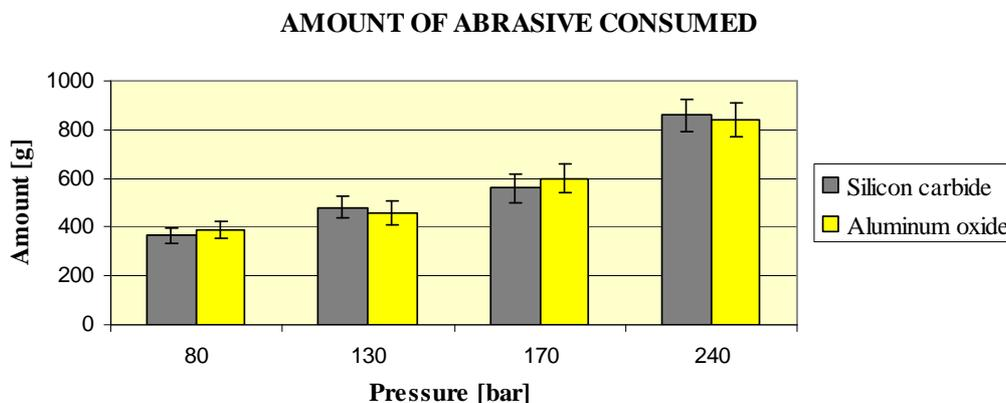
Figure 9. Amount of abrasive consumed in the AJEDM process for the different pressure values, deionized water dielectric fluid
