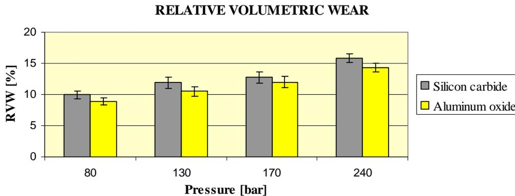
Figure 8. RVW results of AJEDM process for different pressure values with the SiC and Al<sub>2</sub>O<sub>3</sub> 600 mesh, deionized water dielectric fluid
