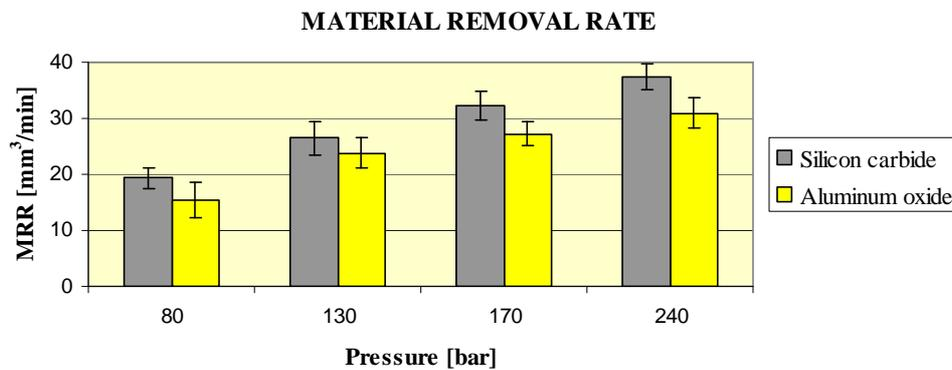
Figure 6. MRR results of AJEDM process on different pressure values with abrasive particles of SiC and  $\text{Al}_2\text{O}_3$  600 mesh, deionized water dielectric fluid
