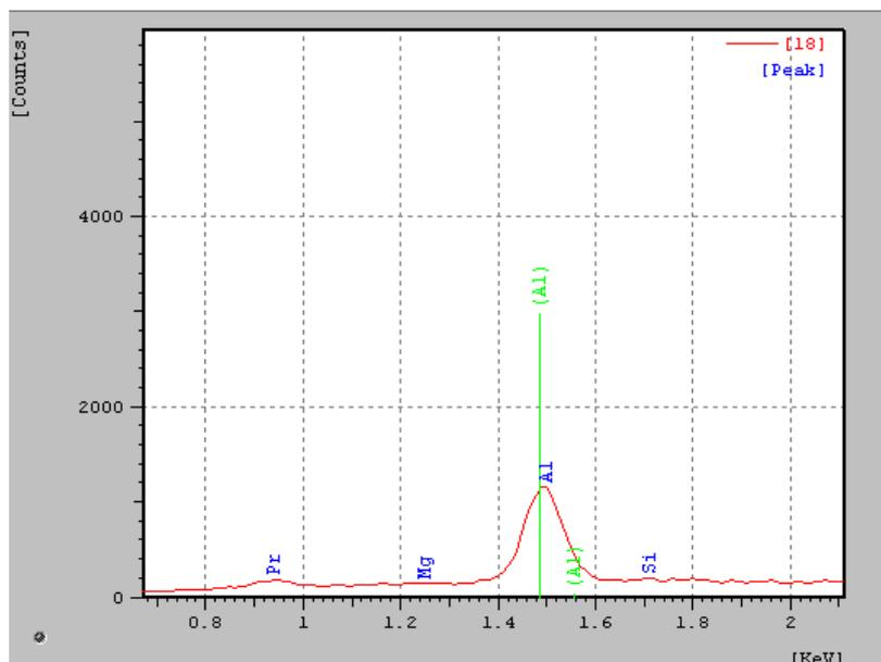
Figure 13. Image of the punctual EDX specter of the particle inserted to the surface machined by AJEDM process using  $\text{Al}_2\text{O}_3$  600 mesh and work pressure of 240 bar
