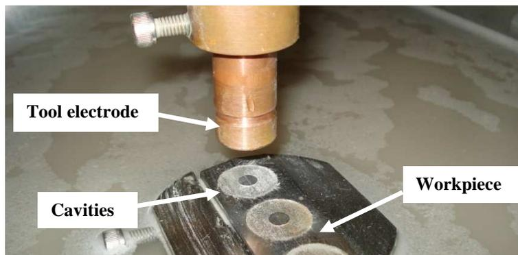
Figure 4. Picture illustrating the tool electrodes and the machined part with the cavities being highlighted
