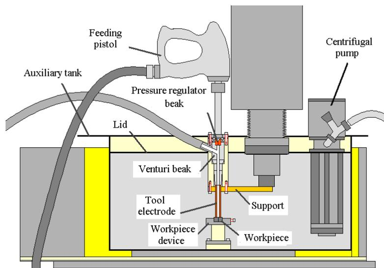
Figure 2. Schematic drawing of the auxiliary tank assembled to the machine
