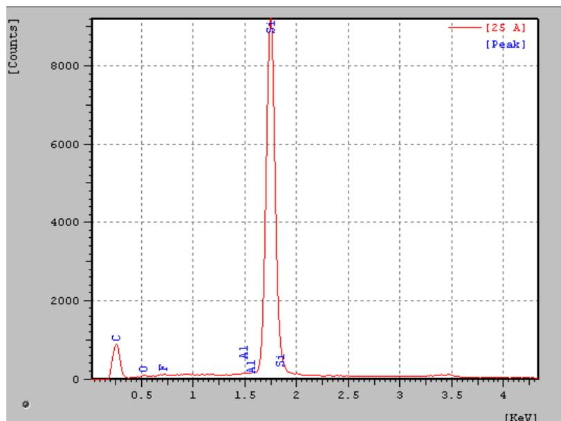
Figure 11. Image of the punctual EDX specter of the particle inserted to the surface machined by AJEDM process using SiC 600 mesh and work pressure of 240 bar
