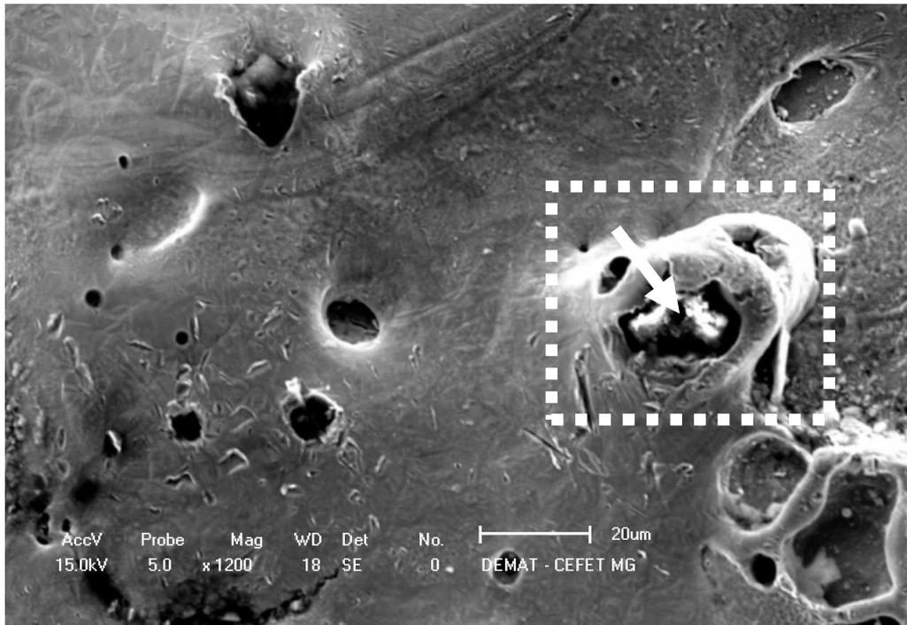
Figure 10. Scanning Electron Microscopy on the surface machined using AJEDM process with SiC 600 mesh and a work pressure of 240 bar
