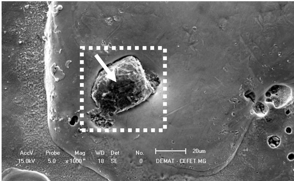
Figure 12. Scanning Electron Microscopy on the surface machined using AJEDM process with  $\text{Al}_2\text{O}_3$  600 mesh and a work pressure of 240 bar
