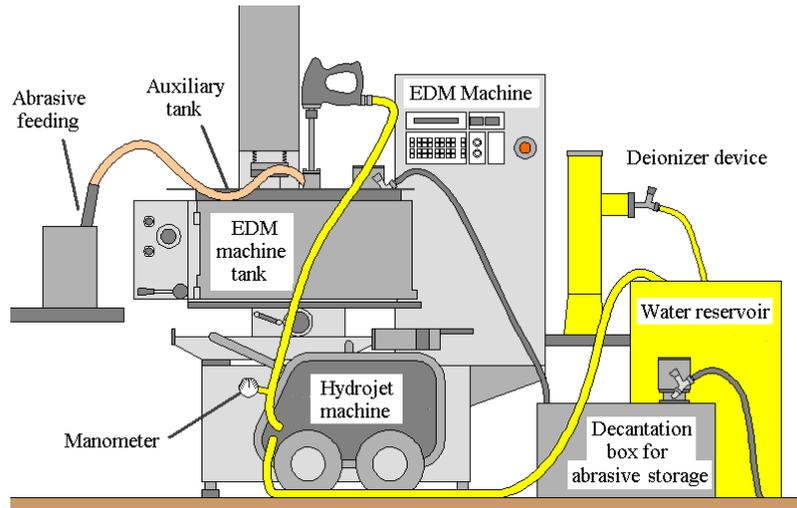
Figure 1. Schematic drawing of the AJEDM process
