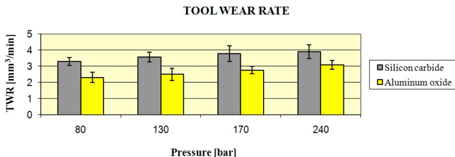
Figure 7. TWR results for the AJEDM process for different pressure values with the SiC and  $\text{Al}_2\text{O}_3$  600 mesh, deionized water dielectric fluid
