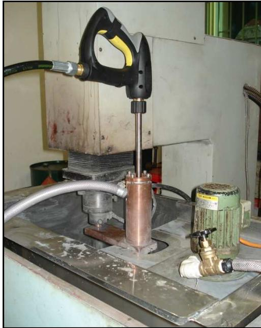
Figure 3. Picture illustrating the adaptations that were made to the EDM machine for the application of the AJEDM hybrid process
