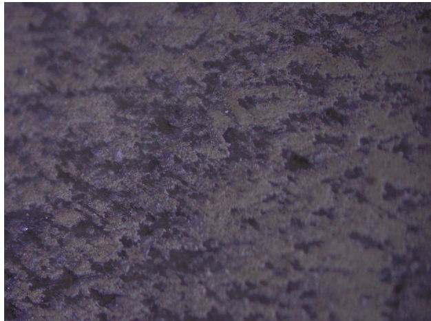
Figure 5. Ceramic submerged in ocean petroleum for 30 days (Magnificatio 200X)
