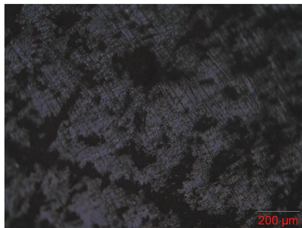
Figure 9. Ceramic submerged in earth petroleum for 45 days (Magnificatio 200X)
