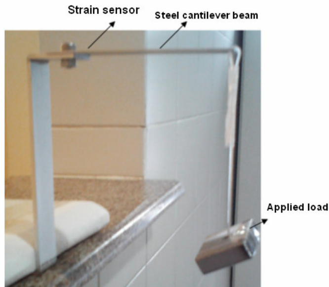
Figure 3. Photograph of the experimental setup for characterization of the strain sensors
