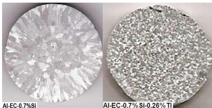
Figure 6 - Macrostructures of the base alloy without additional and modified with Ti content of 0.26%.
