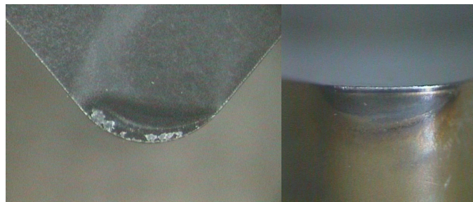
Figure 3. Tool wear on insert KR 3205 when rough turning ADI G2 with low feed rate.
