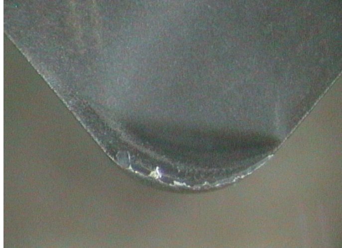
Figure 6. Tool wear on insert KR 3205 when rough turning ADI G2 with high cutting speed.
