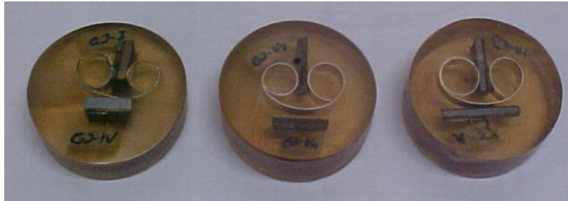
Figure 8. Test specimens ready for metallographic analysis.
