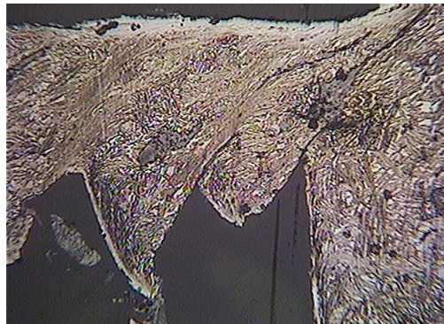
Figure 11. One of the photos made at ADI G2 specimen with 100 m/min showing the plastically induced transformation of the retained austenite to martensite inside the chip.
