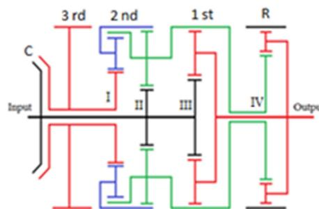
Figure 4. Relationship between the planetary elements
