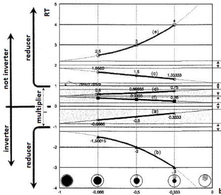
Figure 2. Transmission ratio in function of the basic reason “b” (Adapted from Amaral, D., 2000).
