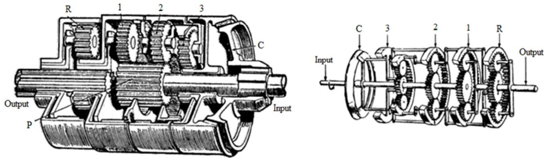
Figure 1. Wilson gearbox (Adapted from Arias Paz, 1958).
