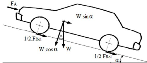
Figure 5. Main resistive efforts of the vehicle, adopted of Ehsani, G., et al. (2005).
