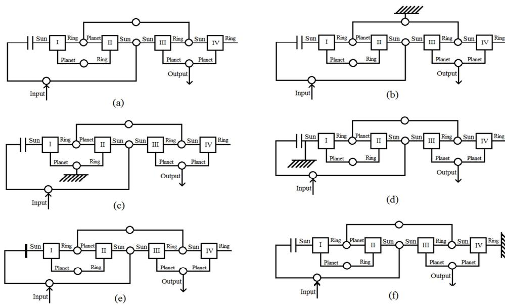
Figure 3. Block diagram of a four speed Wilson Gearbox
