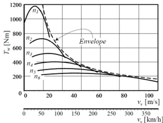
Figure 6. Graph of torque at the wheels in a vehicle with six transmission ratio gearbox (Jazar, R. N., 2008).
