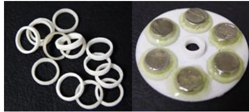
Figure 8. Housing of the magnets removed and the magnets fixed with epoxy resin
