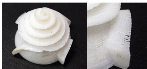
Figure 12. Flaws from the construction process of the rotor
