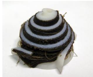
Figure 6. Prototype of the rotor still with the support material not removed.
