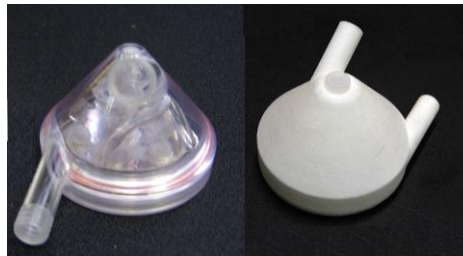
Figure 11. Acrylic prototype and Polyamide prototype
