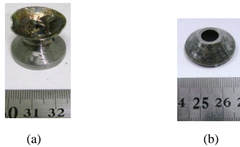
Figure 5. (a) Unfinished final product of the melting. (b) SMA Belleville washer finished.
