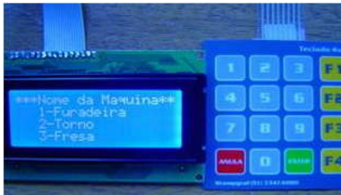
Figure 3. Prototype data collector based on a microcontroller (Leandro et al. , 2006).
