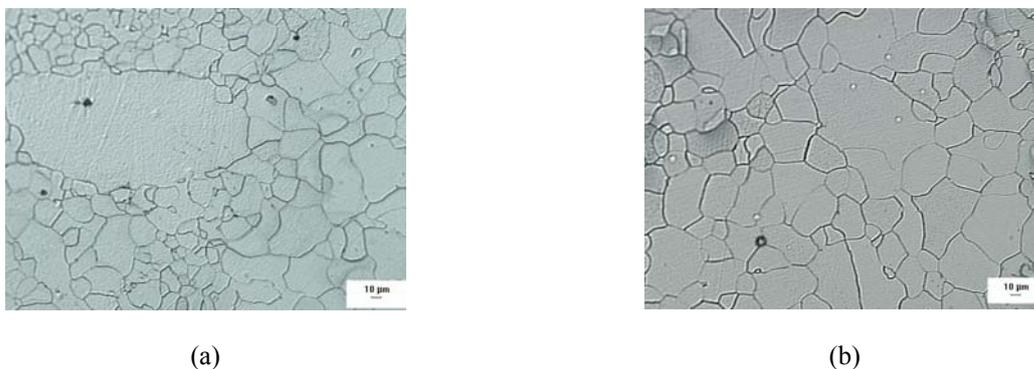
Figure 1. Optical micrography after annealing (a) inside and (b) outside magnetic field. Magnification 200X
