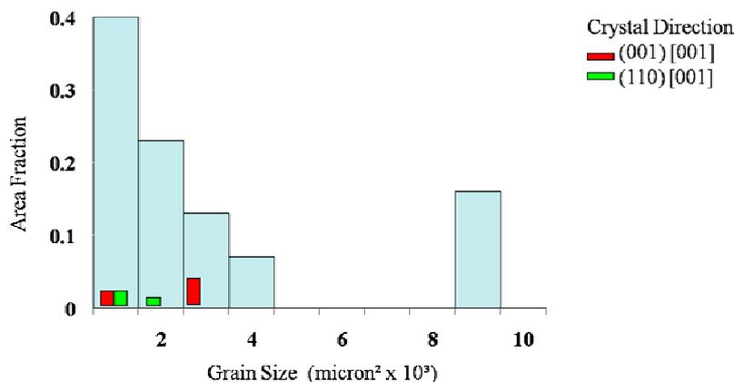
Figure 3. Grain size distribution after annealing outside magnetic field - sample HO810
