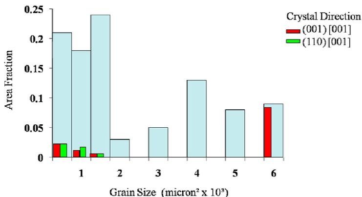
Figure 2. Grain size distribution after annealing inside magnetic field - sample HM810
