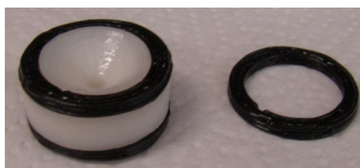
Figure 8 - O-ring made by silicone
