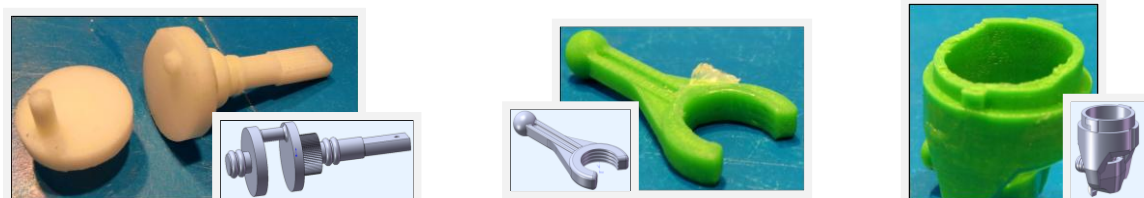
Figure 7 - Breaks due to under sizing, poor lubricating and load in weak resistance direction
