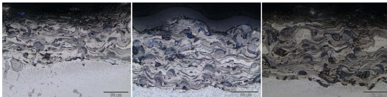
Figure 10 – Optical Microscopy of specimens A1, A2 e A3, Diamalloy 4008NS
