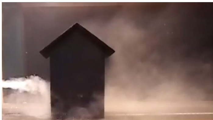
Figure 13. Side view of flow visualization for Building 3 with \theta = 0^\circ and Re = 6055.
