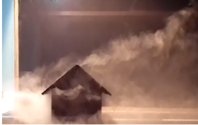
Figure 5. Side view of the flow visualization for Building 2 with \theta = 0^\circ and Re = 1646 .
