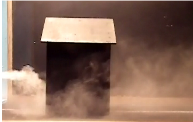
Figure 20. Side view of flow visualization for Building 3 with \theta = 90^\circ and Re = 16876 .
