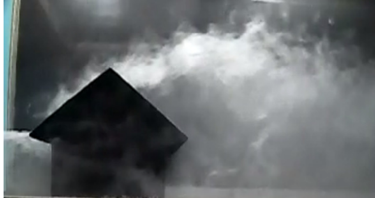
Figure 11. Side view of the flow visualization for Building 2 with \theta = 0^\circ and Re = 6055.
