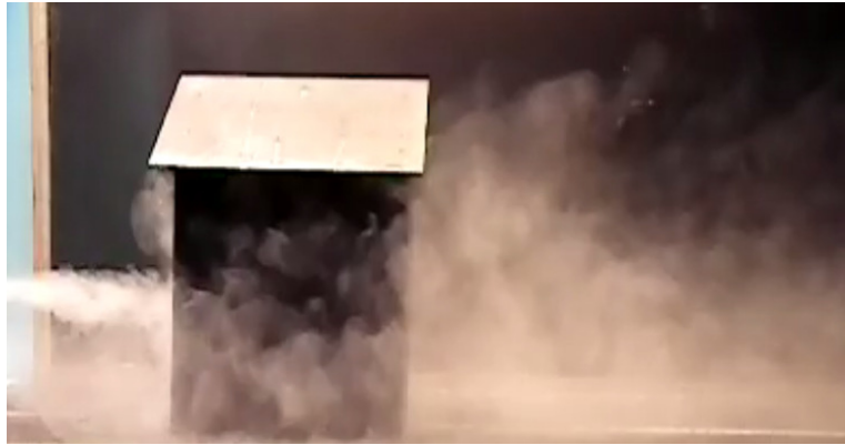
Figure 8. Side view of flow visualization for Building 3 with \theta = 90^\circ and Re = 1646 .
