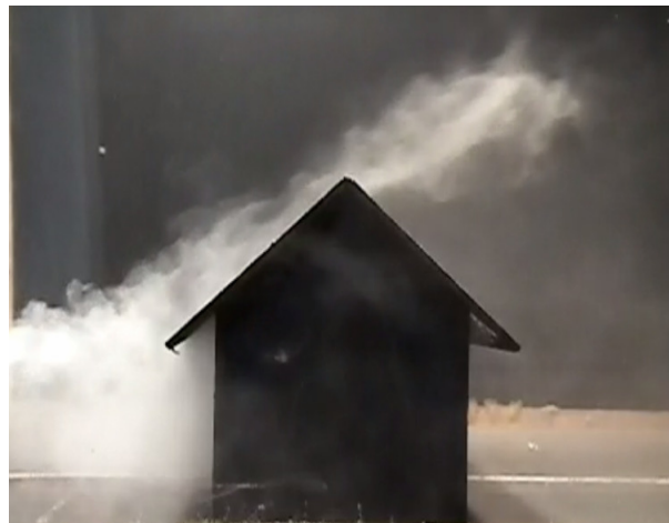
Figure 16. Side view of flow visualization for Building 2 with \theta = 0^\circ and Re = 16876 .
