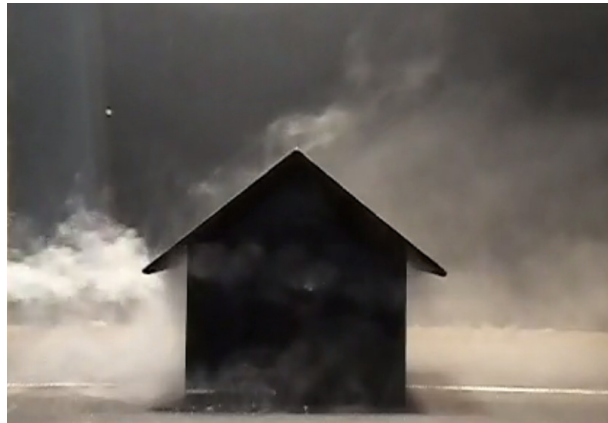
Figure 15. Side view of flow visualization for Building 1 with \theta = 0^\circ and Re = 16876 .
