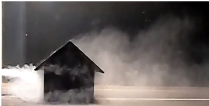
Figure 9. Side view of flow visualization for Building 1 with \theta = 0^\circ and Re = 6055 .
