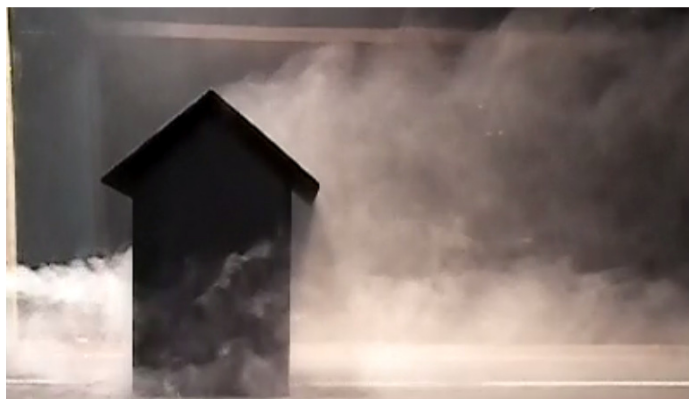
Figure 7. Side view of the flow visualization for Building 3 with \theta = 0^\circ and Re = 1646 .
