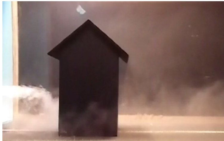
Figure 17. Side view of flow visualization for Building 3 with \theta = 0^\circ and Re = 16876 .
