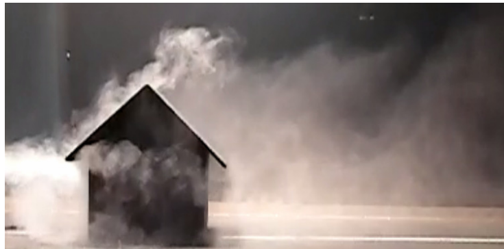
Figure 3. Side view of flow visualization for Building 1 with \theta = 0^\circ and Re = 1646 .
