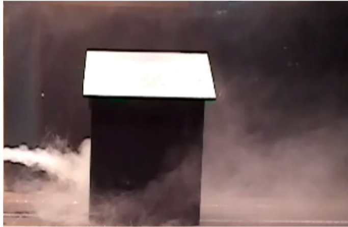
Figure 14. Side view of flow visualization for Building 3 with \theta = 90^\circ and Re = 6055 .
