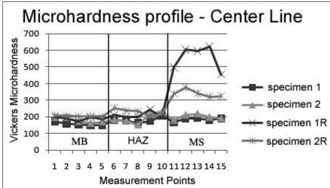
Figure 3 – Graph of microhardness profile of the centerline of the specimens.
