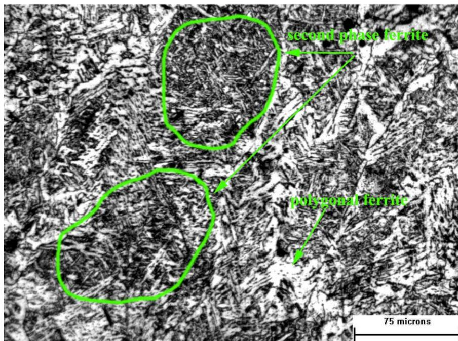
Figure 8 – Micrograph of the weld metal of the specimen welded with MIG/MAG process. Etching – Nital 2%.
