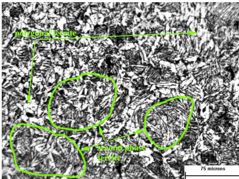
Figure 5 – Micrograph of the heat affected zone of the specimen welded with SMAW process. Etching – Nital 2%.
