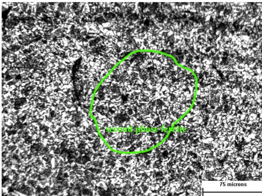
Figure 7 – Micrograph of the heat affected zone of the specimen welded with MIG/MAG process. Etching – Nital 2%.
