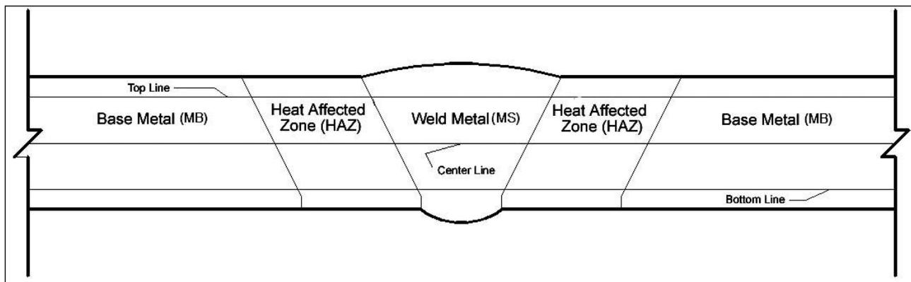
Figure 1 – Diagram of the lines of microhardness measuring.
