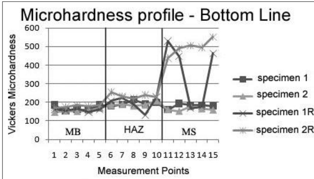
Figure 2 – Graph of microhardness profile of the bottom line of the specimens.
