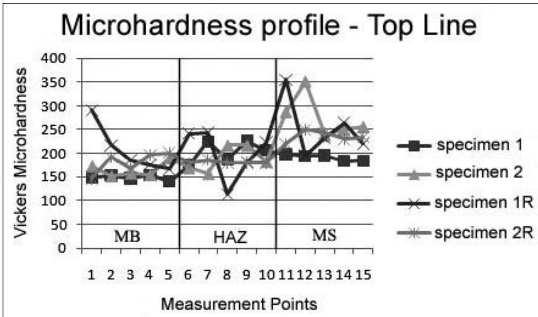
Figure 4 – Graph of microhardness profile of the top line of the specimens.
