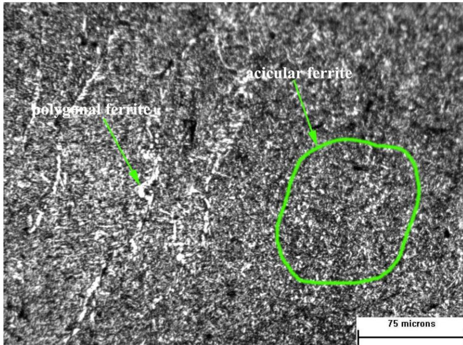
Figure 6 – Micrograph of the weld metal of the specimen welded with SMAW process. Etching – Nital 2%.
