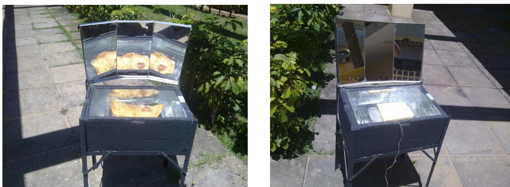
Figure 2. Solar oven / cooker under test.
