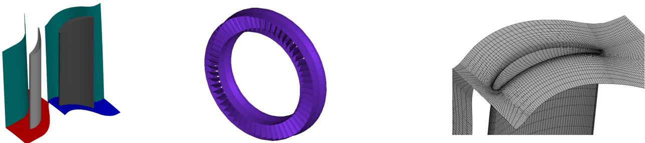
Figure 1. 3D view and the mesh at rotor casing of the single-stage axial-flow turbine
