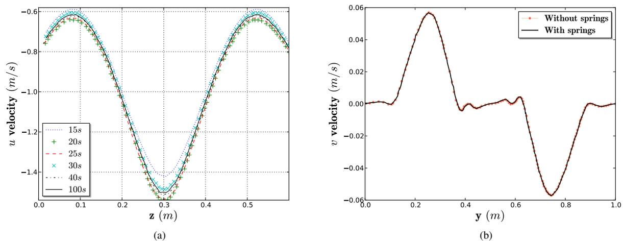
Figure 6: Velocity profiles in the fluid-structure interaction case; (a)  $u$  velocity in the center of the Taylor vortices and (b) steady state  $v$  velocity comparison with the classical Taylor-Couette flow.
