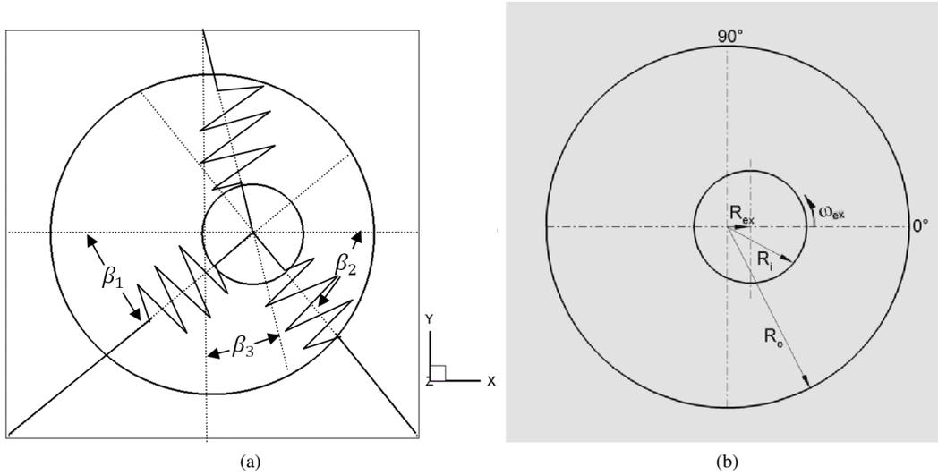
Figure 2: Schematics of the inner cylinder (a) supported by three strings and the corresponding  $\beta$  angles and (b) at rest.
