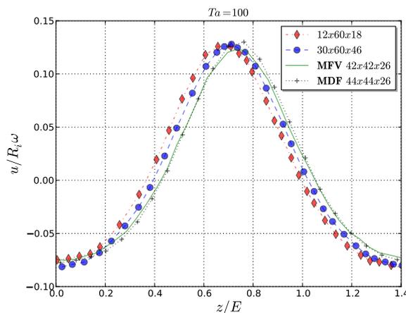
Figure 3: Non-dimensional radial velocity distribution along axial direction to  $Ta = 100$ .
