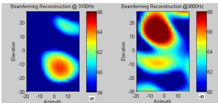
Figure 7. Reconstruction of the Beamforming patterns for two loudspeakers case.
