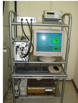
b) Acquisition hardware, signal generator, amplifier, power source and interface
