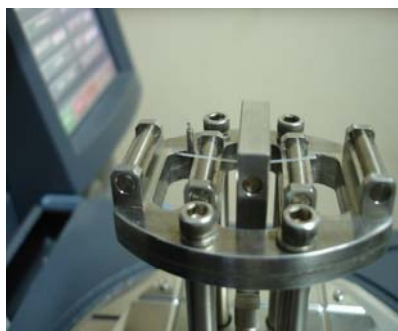
Figure 4 - Test setup for three-point bending creep test
