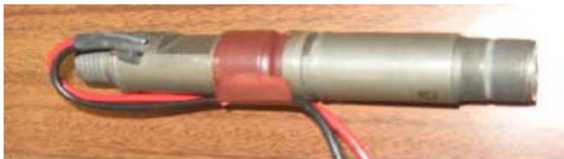
Figure 7 – Piezoelectric actuated diesel injector actuator. The injection head is not present.
