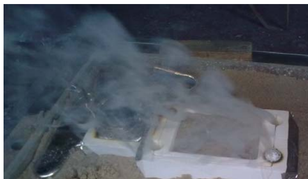
Figure 4 - Excessive moisture and smoke being released from a 3D Printed Rapid Mould
