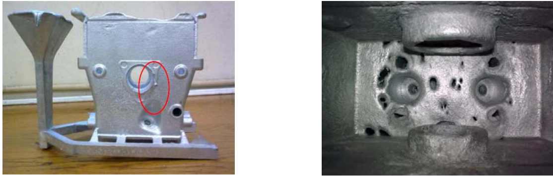
Figure 5 - Casting defects in an aluminum part originated by excessive moisture and smoke release: Outer walls (left) and inner walls (right) aspect.
