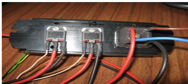
Figure 12 – Rectifier bridge and IGBT arrangement
