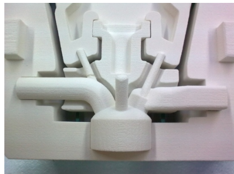
Figure 3 - Combustion chamber, inlet and exhaust passages inner core (left) placed in position (right)
