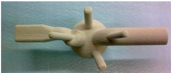
Figure 3 - Combustion chamber, inlet and exhaust passages inner core (left) placed in position (right)
