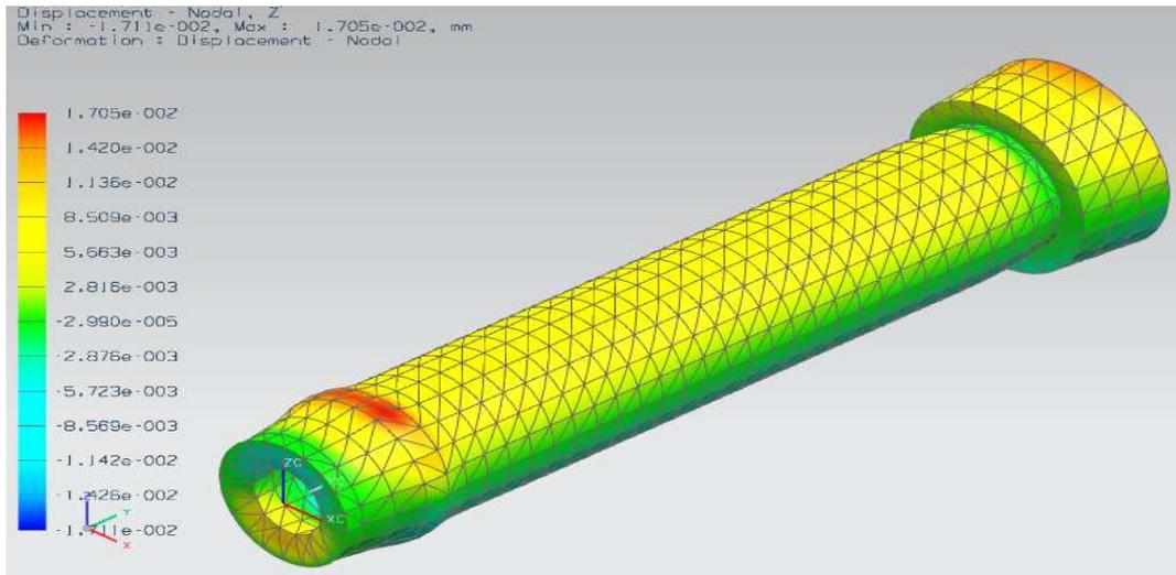
Figure 12. Simulation to determine the displacements in z direction.
