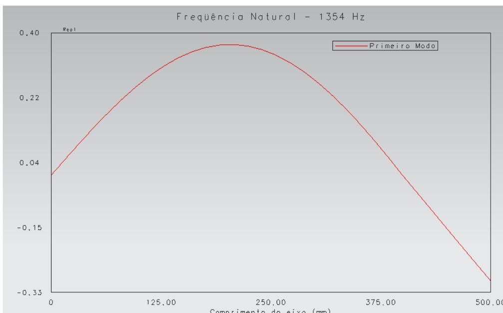
Figure 4. First vibration mode, 1354 Hz
