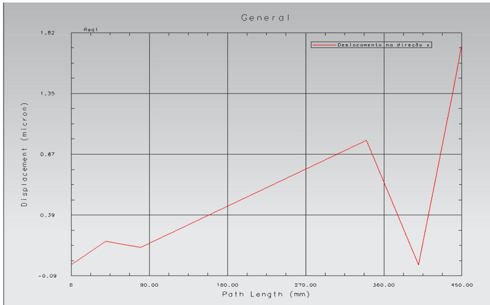
Figure 3. Elastic curve of the spindle in the x direction
