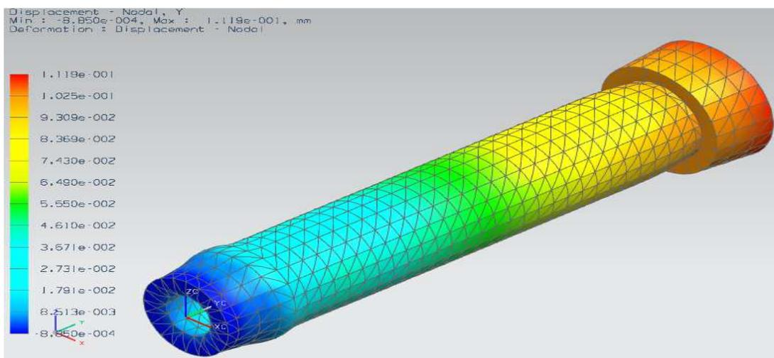
Figure 11. Simulation to determine the displacements in y direction.
