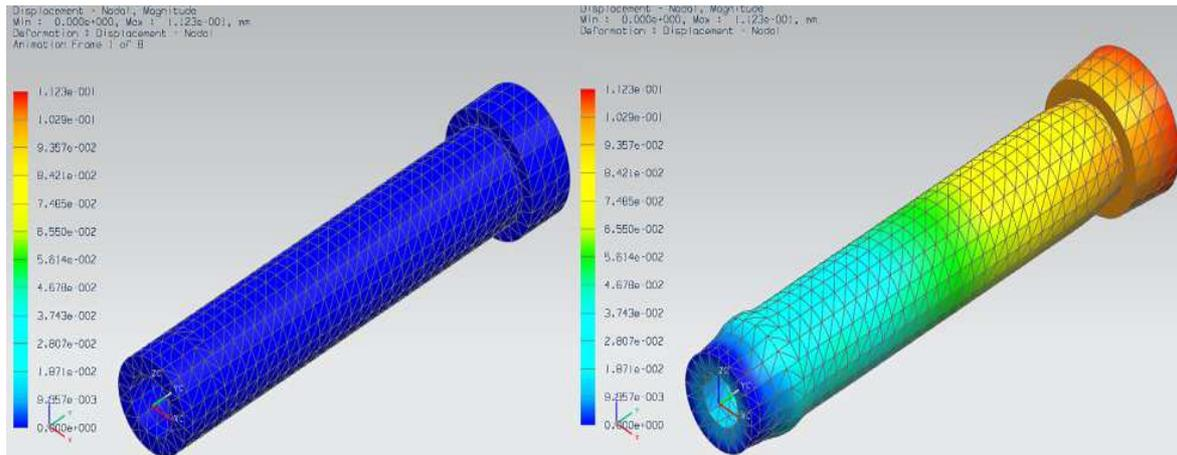
Figure 9. Thermal displacement of spindle subjected to certain temperatures.
