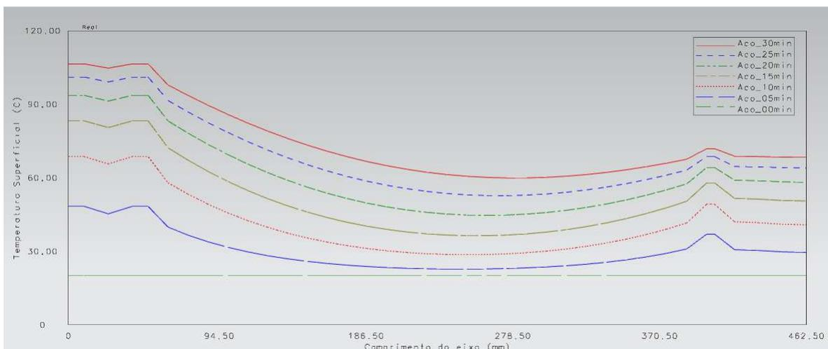
Figure 7. Surface temperatures of the spindle in steel during the first thirty minutes of operation.
