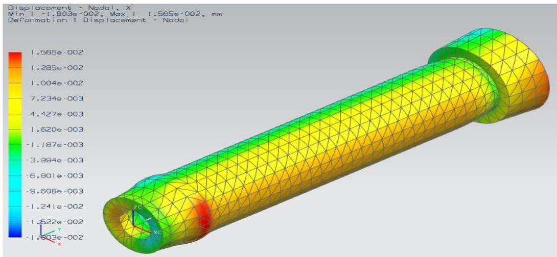
Figure 10. Simulation to determine the displacements in x direction.
