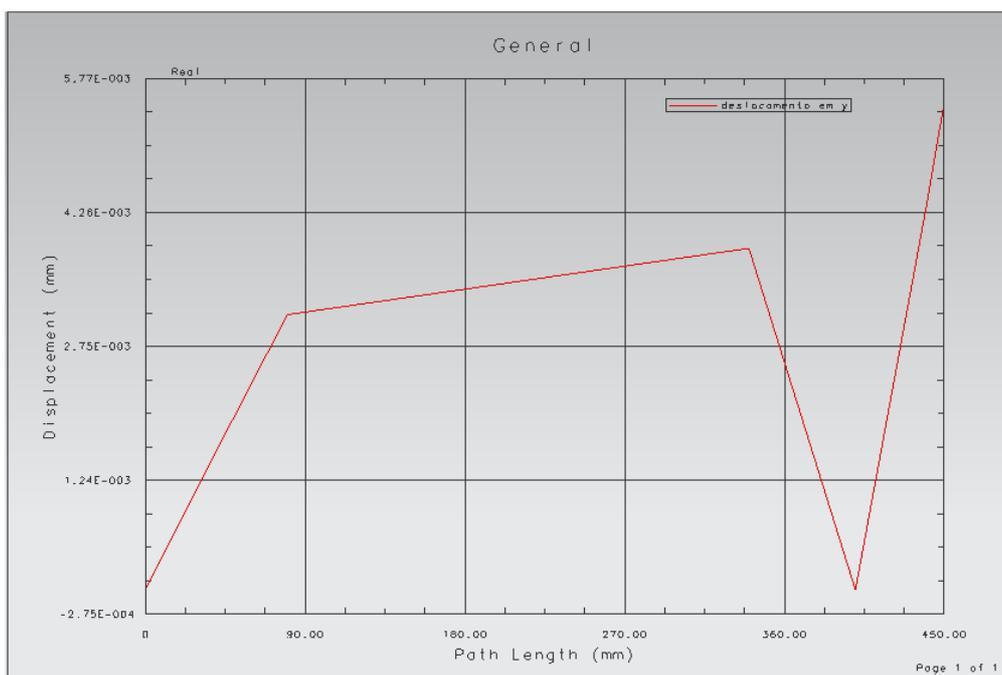
Figure 3. Elastic curve of the spindle in the y direction
