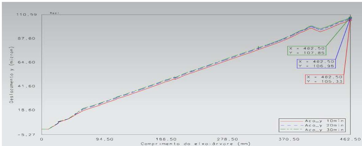
Figure 13. Surface displacement of the spindle in the y direction at t = 10 min, 20 min and 30 min.
