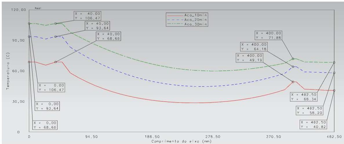
Figure 8. Distribution of surface temperature of steel at  $t = 10$  min, 20 min and 30 min.
