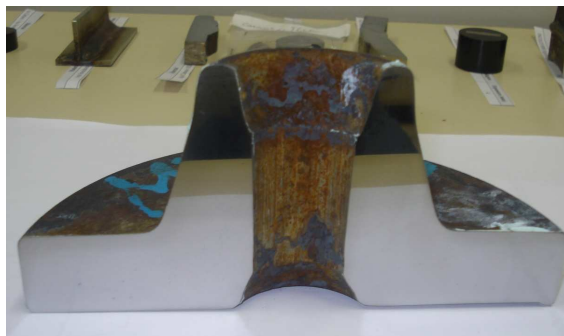
Figure 2. Forged in cutting, properly polished to macrography
