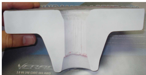
Figure 9. Revelation of the forged piece derived from ingot casting with electromagnetic stirring without apparent defects
