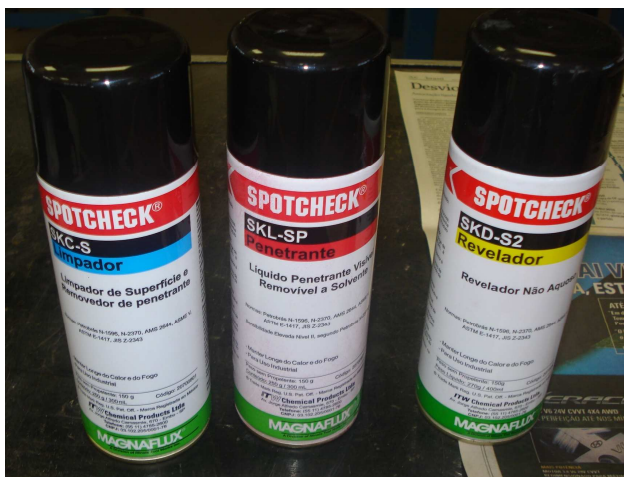
Figure 7. Products used in the penetrating liquids non-destructive test
