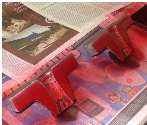
Figure 8. Penetrant in all parts of the section
