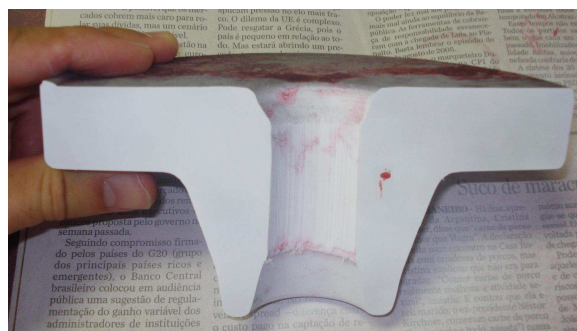
Figure 10. Revelation of the forged piece derived from ingot casting without electromagnetic stirring with discontinuity found
