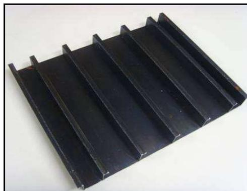
Figure 2: Small scale stiffened panel
