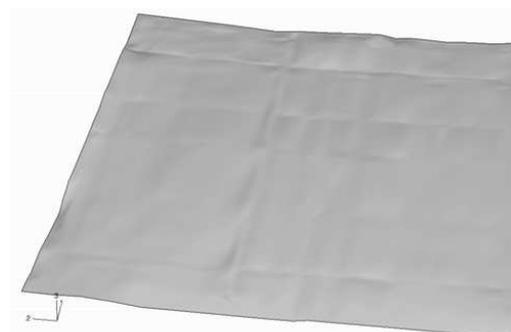
Figure 15: Plate with measured imperfection distribution (amplified 20 times)
