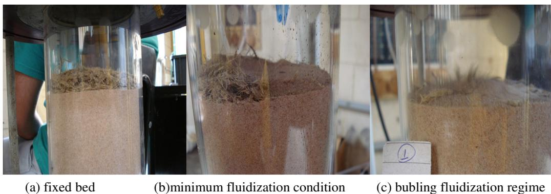
Figure 3. Fluidization regimes at bed containing the bagasse/sand mixture
