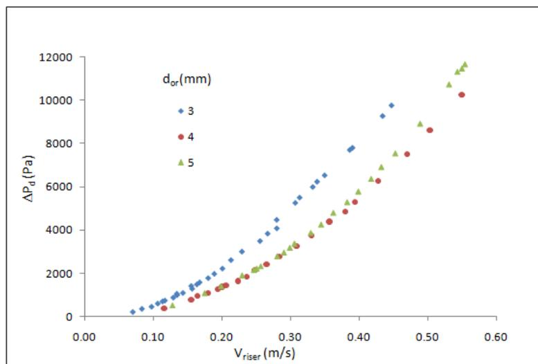
Figure 4. Gas distributor pressure drop ( $\Delta P_d$ ) for tested orifices diameters (no solid material inside the riser).
