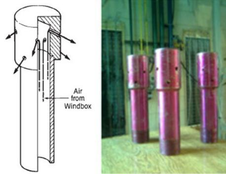
Figure 2. Tuyeres or nozzles type gas distributor
