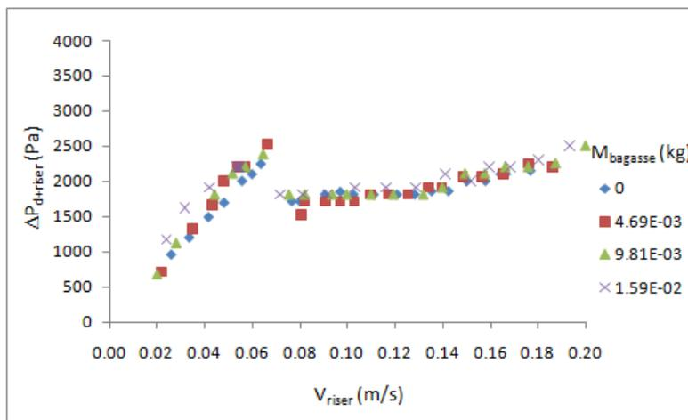
Figure 8. Bed pressure drop plus distributor pressure drop ( $\Delta P_{d+riser}$ ) for 5 mm orifice diameter at the nozzle
