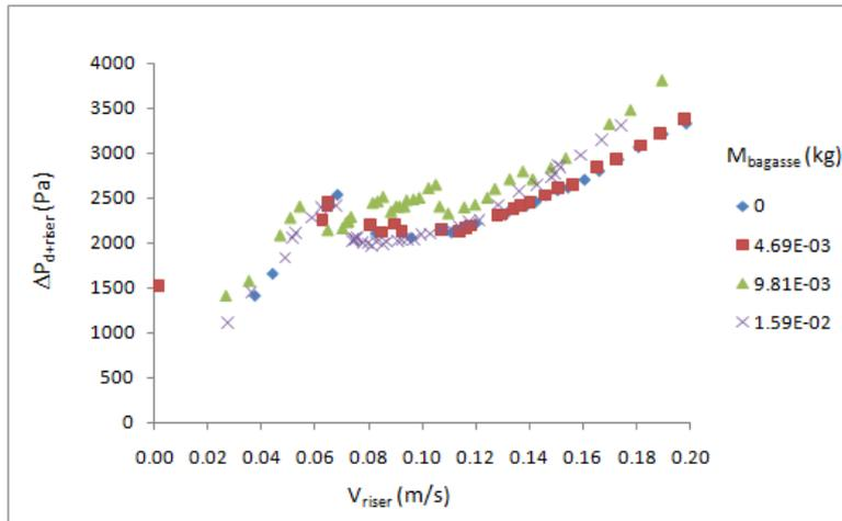
Figure 6. Bed pressure drop plus distributor pressure drop ( $\Delta P_{d+riser}$ ) for 3 mm orifice diameter at the nozzle
