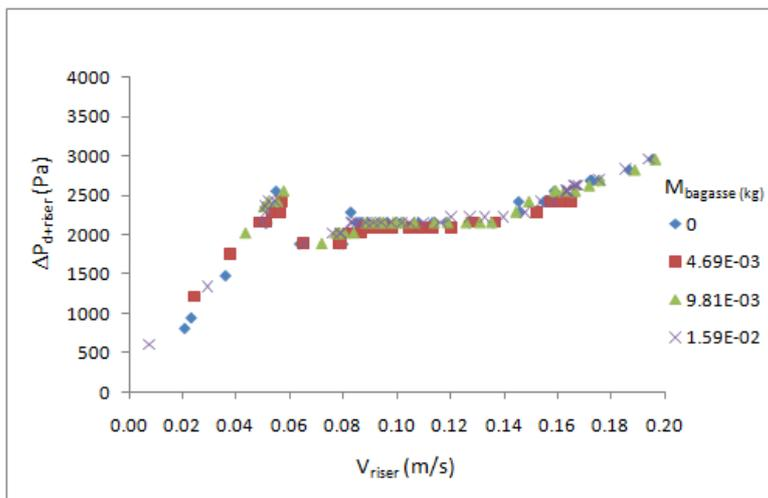
Figure 7. Bed pressure drop plus distributor pressure drop ( $\Delta P_{d+riser}$ ) for 4 mm orifice diameter at the nozzle
