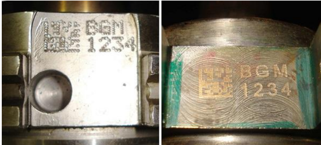
2a – Micropunching engraving
