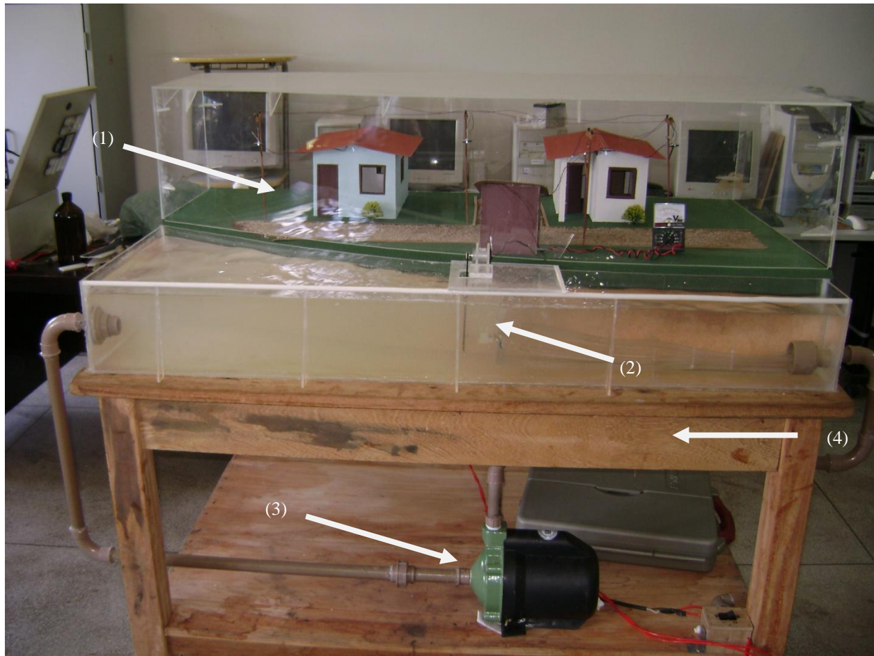
Figure 3. Maquete (1), tank (2), hydraulic system (3), stand (4)
