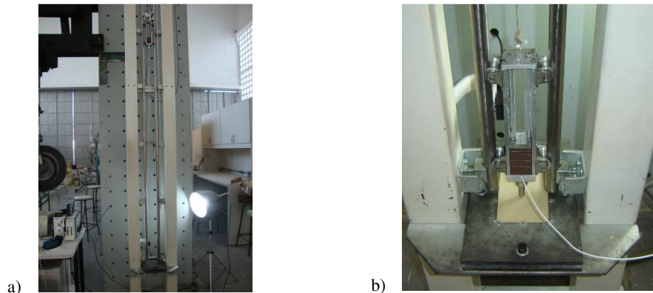
Figure 2 - a) Test Machine; b) Impact test dispositive.
