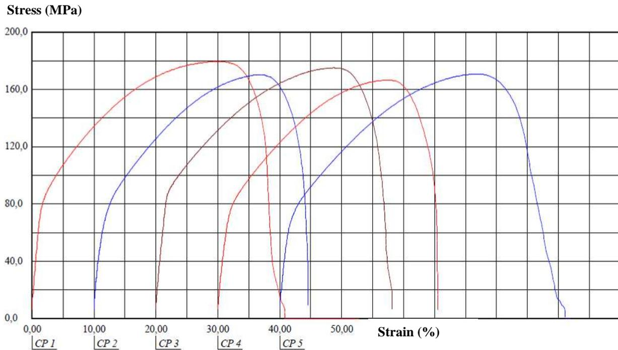
Figure 6. Stress-strain curves of five diffusion bonded specimens submitted to tensile tests.
