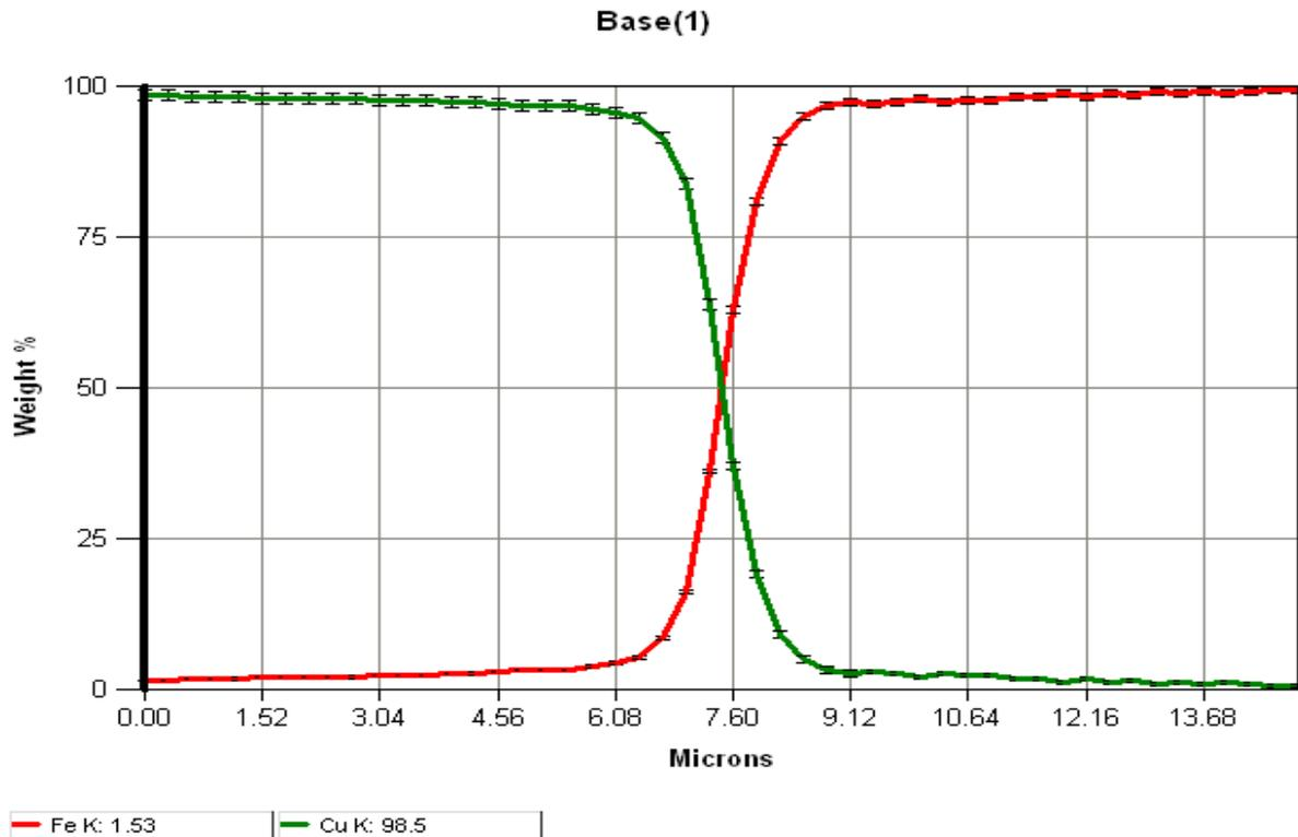
Figure 3. EDS diffusion analysis on interface of copper and stainless steel joint.
