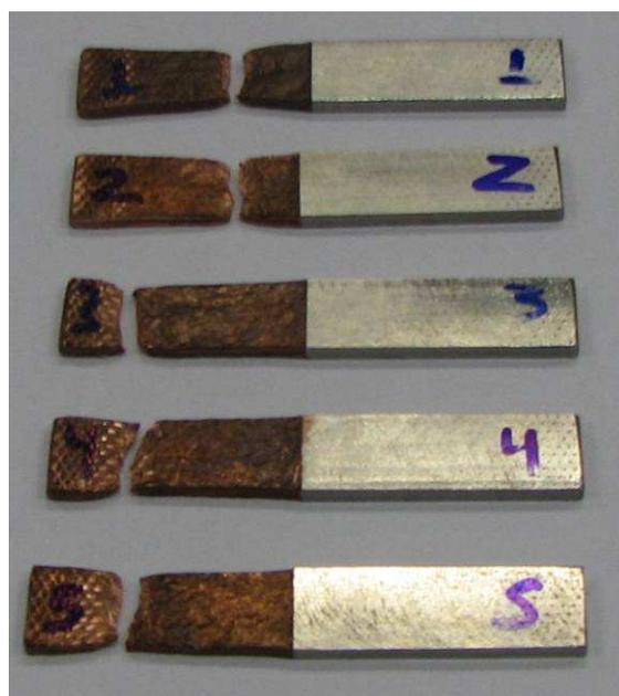
Figure 7. Diffusion bonded specimens after tensile test, resulting in a rupture in copper base material.
