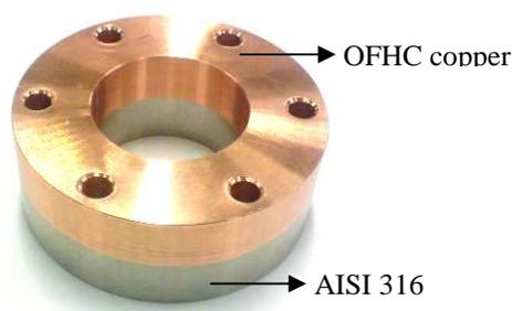
Figure 2. Diffusion bonded AISI 316L to OFHC copper specimen machined for leak test.
