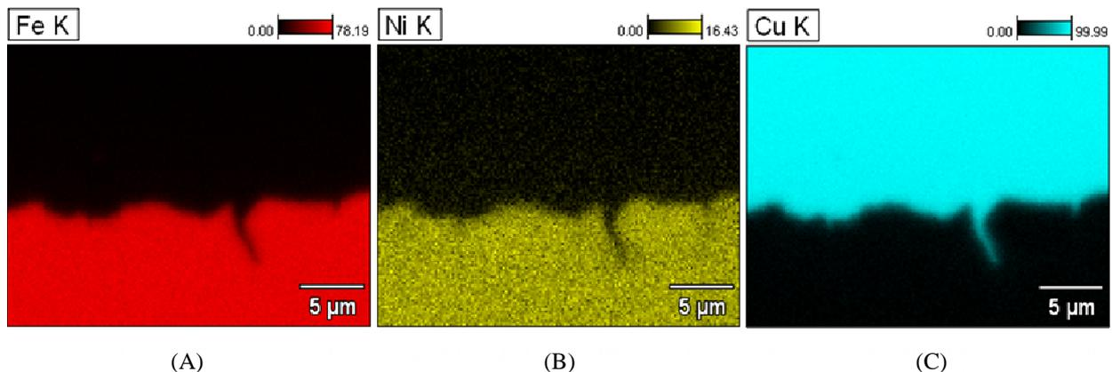
Figure 4. EDS of (A) Fe (red) and Cu (black); (B) diffusion between Ni and Cu and (C) detail of Cu in the interface.
