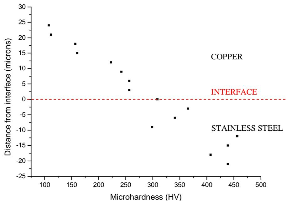
Figure 5. Microstructural characterization and microhardness profile across the diffusion interface.
