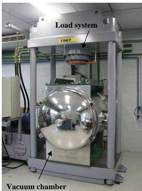
Figure 1. Experimental set up and diffusion bonding furnace.
