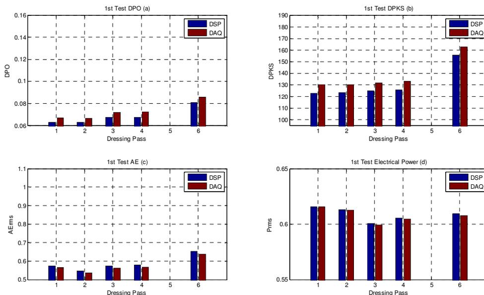
Figure 4. First pass (a) Comparison of Static DPO. (b) Comparison of Static DPKS. (c) Comparison of the mean of acoustic emission signal. (d) Comparison of the mean of electric power signal.
