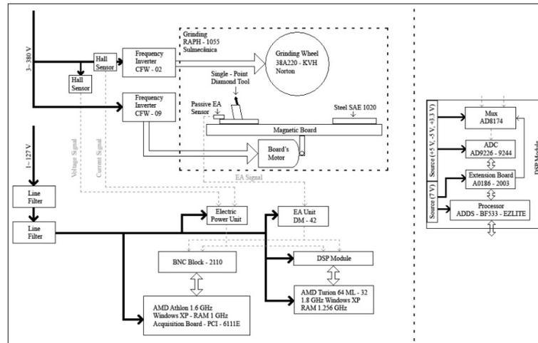
Figure 1. Schematic diagram of the test bench
