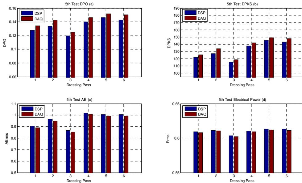
Figure 6. Fifth pass (a) Comparison of Static DPO. (b) Comparison of Static DPKS. (c) Comparison of the mean of acoustic emission signal. (d) Comparison of the mean of electric power signal.
