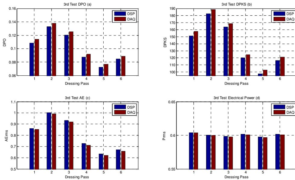
Figure 5. Third pass (a) Comparison of Static DPO. (b) Comparison of Static DPKS. (c) Comparison of the mean of acoustic emission signal. (d) Comparison of the mean of electric power signal.
