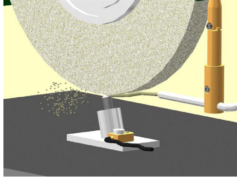
Figure 2. Schematic assembly of the dressing process with the Acoustic Emission Sensor
